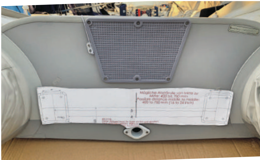
Stick the prepared drilling template to the back of the dinghy.
