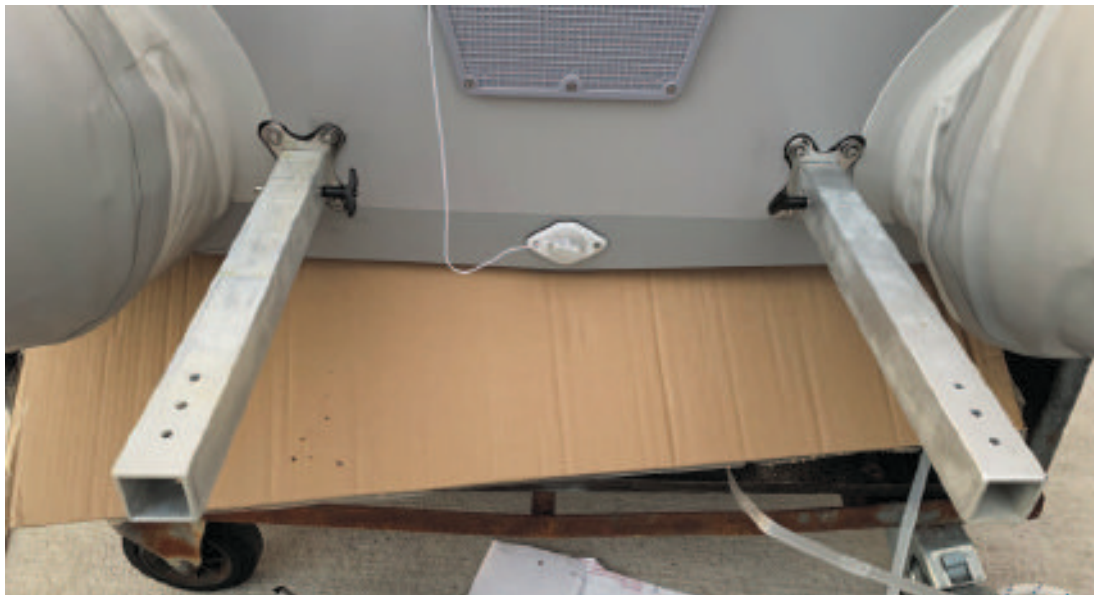
Installation at dinghy is completed.
